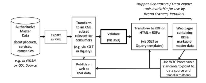
Figure 1: For master data that is already available as XML, it may be sufficient to rely on XML Schema (XSD) to validate and to use W3C Provenance standards to refer back to the XML source data and the transformations (e.g. XSLT or XQuery templates) that generated the RDF output or HTML + RDFa markup.
